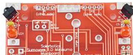
Steps 15, 16 & 17: IR Sensors, Caps, and LEDs
