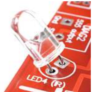
IR LED Installation
