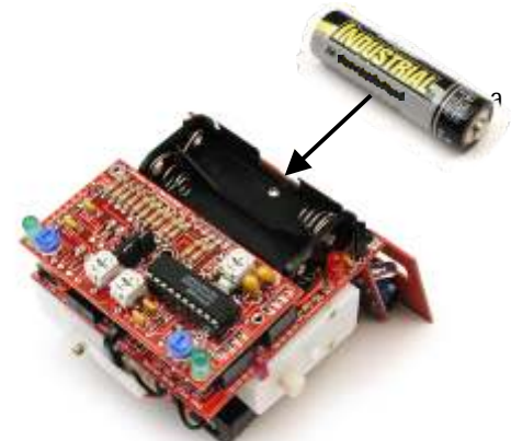
Step 13: Install brainboard Step 14: Install batteries
