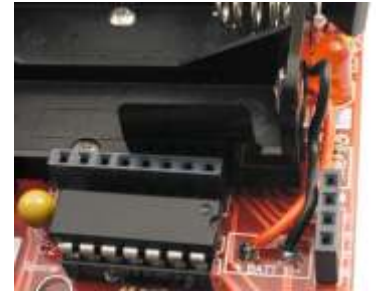
2AA Battery Pack Installed and Wired
