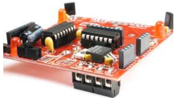
Steps 19: Terminal Blocks Installed
