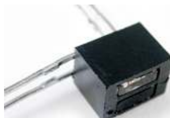
...then fold the leads on the dimple side down flat to the sensor...
