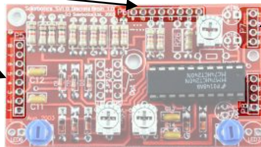
Steps 46 & 47: 8 and 4 pin installation UNDERNEATH!
