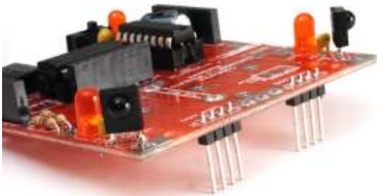
Steps 18: Front Pins Installed
