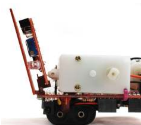
Test installation of front edge sensor board
