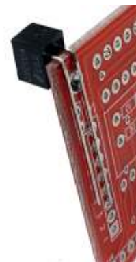
...and use the circuit board as a spacer to fold over the other two lead over the first pair.
