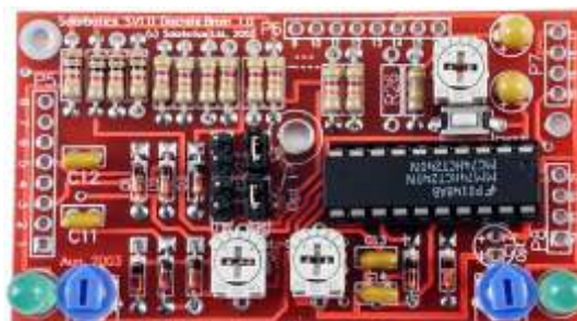
Step D: Install the jumpers on the pin pair on the 'MS' side (right side)
