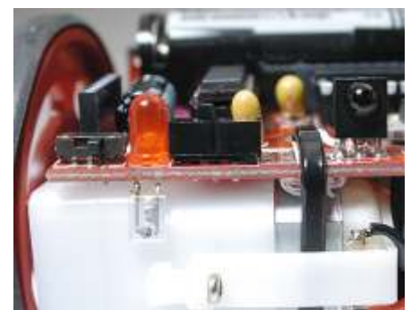
Step 4 (Opt.): Install IR Emitter below LED3
